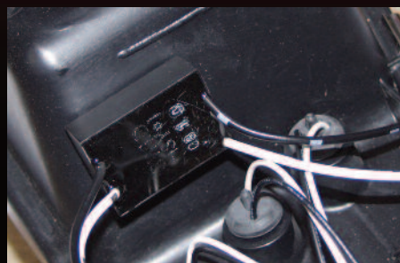
Resistor box for angel eye LED bulbs
