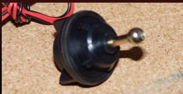
Pivot after removal from new headlight unit.
