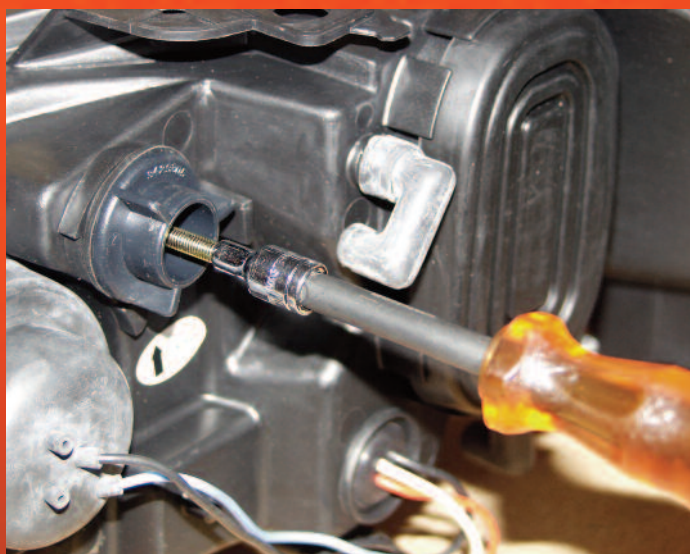
Screw pivot adjuster all the way in before removing
