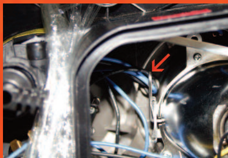
Adjusting lever behind dipped beam unit for setting lights for left- or right-hand drive use.
