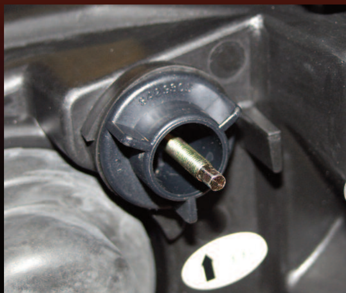
Pivot on rear of new headlight unit.
