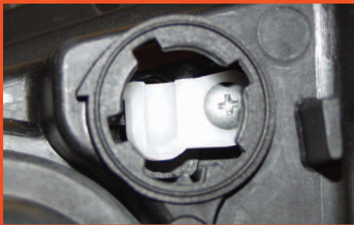
Nylon socket showing slot for ball on motor shaft.
