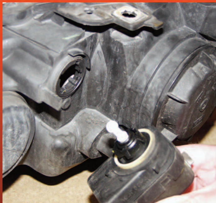
Adjustment motor removed from old headlight unit, locating lugs are clearly visible.
