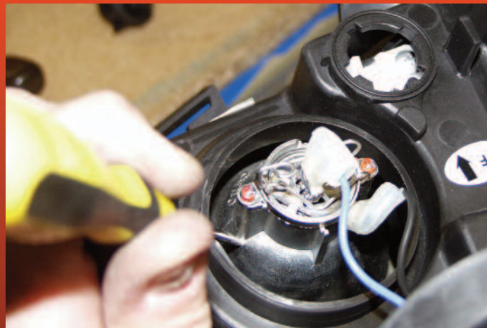
Holding the frame in position so that the nylon socket is accessible.
