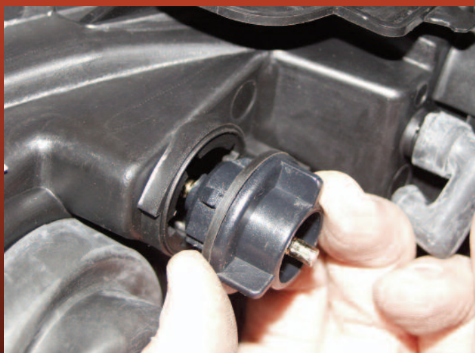
Removing the pivot from the new headlight unit
